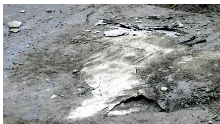
图5 岩爆现象 Fig.5 Image of rockbursting
